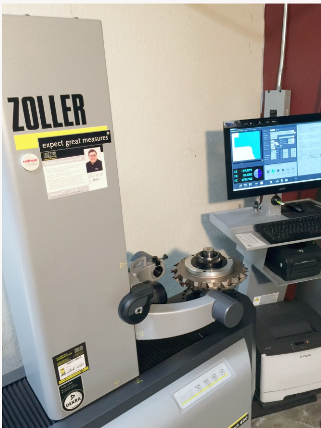
Tool measurement after service to ensure accuracy at Surrey Precision Tools, Inc.
